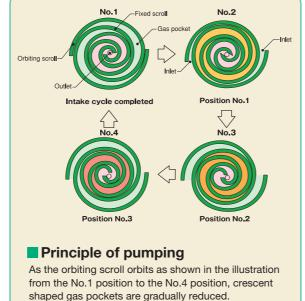
At the last stage compressed gas is exhausted through
